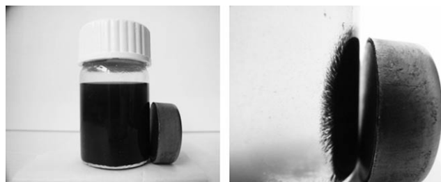
Figure 4. Magneto filtration of finely dispersed superparamagnetic 1Mo@SMNP nanoparticles ( left : shortly after the application of the magnet; right : 2 min later)
